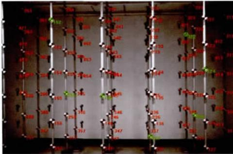
Fig. 4 Camera calibration range
